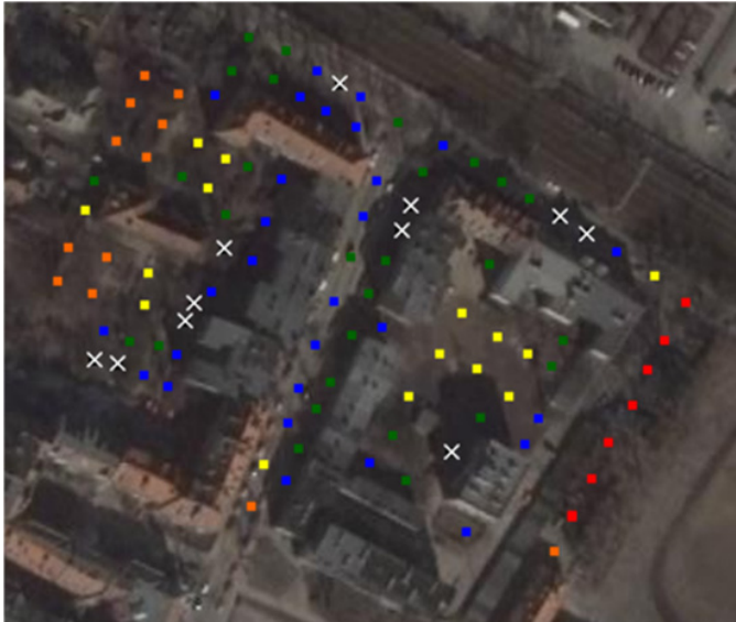
Fig. 2. WiMAX coverage white spot effect. Measurements taken in testbed employing a single BS working in 3.5 GHz band. Colors show stable modulation chosen by a terminal: x - no connectivity, blue - BPSK, green - QPSK, yellow - QAM16, orange - QAM64 1/2, red - QAM64 3/4.
