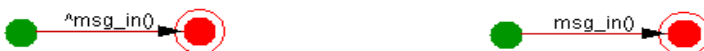
Fig. 7. Statecharts diagrams of send_receive1 or send_receive2 Initiator conversation (the left statecharts diagram) and Responder conversation (the right statecharts diagram).
